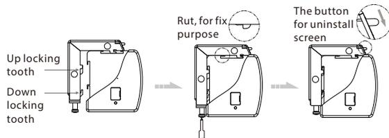
Note: When taking off screen, loosen the bottom screw first and push the top loosen button, then you can easily take the screen off, as above figure:
