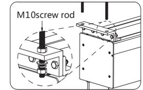
Screw mounting: measure the distance between the four oblong holes on the left and right hanging plates respectively, install M10 screw rods directly above the corresponding holes to connect the left and right hanging plates, install an adjustable hook on the middle of the screen to connect the middle hanging plate, and adjust the screws The position of the screen to make the screen to a horizontal state, complete the installation of the screen.
