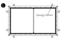
Before assembling the outer black frame, place the sponge cushion under the assembled screen as per the diagram
