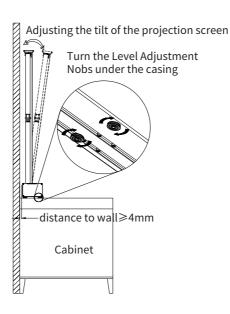
c.Adjust the T-Nuts on the Adjustable Bracket so that they are parallel with the wall (see diagram), place the projection screen on the Adjustable Brackets, adjust the projection screen horizontally to the desire position, tighten the T-Nuts from under the Adjustable Brackets to lock in place. (T-Nuts are installed for front installation in default, user can install the T-Nuts to the Reverse Mounting Holes when needed for reversed installation)
