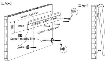
a. Flip the screen to ensure the correct orientation (for ultra-short-throw anti-glare screens). Install S6 in the upper frame slot (note that the hook should face the back). The installation spacing A = 0.52 \* L.
