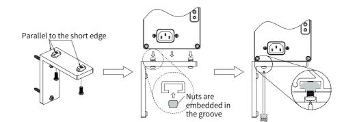
This Right-Angle Bracket is designed with two connecting surfaces, A and B, to adapt to different installation environments. Users need to switch the installation method according to different installations (see the table below).
