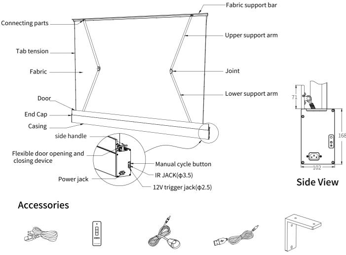
■ Power cable 1pcs ■ IR remote control 1pcs ■ IR receiver 1pcs ■ 12V trigger cable 1pcs ■ Right-Angle Bracket 2pcs
