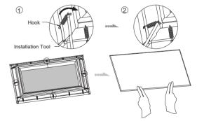
Note: If there is some wrinkles appear, please wear the provided gloves and use fingers to gently press and move on edge area of screen material by left hand to the left side and right hand to the right side.
