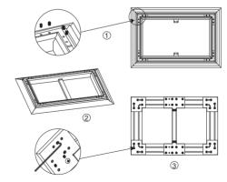
If the screen you purchased is a woven acoustic screen, you must put the black Non woven fabric on the front of the aluminum frame before installing the screen, as shown in Figure 4.
