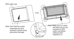
• Use the bigger hook of spring to hitch tension rod from the hole of screen material one by one. Use hook hand to drag the small hook of spring to hitch the slot of frame to tension the screen material. Please start to hitch the frame from the middle position to two sides (left and right) for balance of tension. Please see below:
