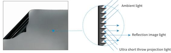
②The screen adpots the splicing process, and the splicing line has a certain curvature due to the source of upper and lower tension, which does not affect the actual projected picture. which is a normal phenomenon.
