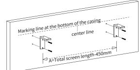
c.Take the M5 boat-shaped nut and M5\*12 screw, connect them to the mounting bracket (keep them loose, do not tighten), adjust the four nuts to be parallel to the short edge of Right-Angle Bracket. Lift the screen, align the bottom groove with the protruding M5 Boat-Shaped Nut, gently lower screen so that all the nuts are embedded in the groove, move the screen left or right to the ideal position, then tighten the screws to secure the screen.
