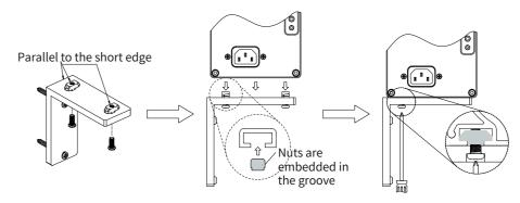
This Right-Angle Bracket is designed with two connecting surfaces, A and B, to adapt to different installation environments. Users need to switch the installation method according to different installations (see the table below).
