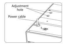
White button Retracted height(lower limit) ে Clockwise Down G Counterclockwise Up
