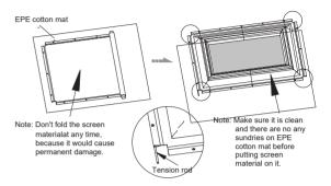
Use the bigger hook of spring to hitch tension rod from the hole of screen material one by one. Use hook hand to drag the small hook of spring to hitch the slot of frame to tension the screen material. Please start to hitch the frame from the middle position to two sides (left and right) for balance of tension. Please see below:
