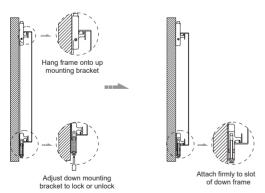
For uninstall of screen, unscrew down mounting brackets till it is loosen from slot of down frame. Lift the screen lightly to make it go off upper mounting bracket and finish uninstall.
