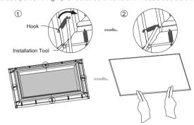
Note: If there is some wrinkles appear, please wear the provided gloves and use fingers to gently press and move on edge area of screen material by left hand to the left side and right hand to the right side.
