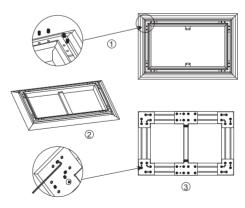
If the screen you purchased is a woven acoustic screen, you must put the black Non woven fabric on the front of the aluminum frame before installing the screen, as shown in Figure 4.
