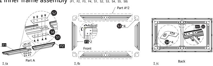
a. Take components F1 and F2 and place them left and right respectively, merging the two vertical notches. Use M5\*8 screws to tighten S1 and S2 onto S8, completing the assembly of component A.
