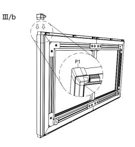
a. Raise the screen, rotate F5 to the correct direction, align with the installation slot of P2, and press down slightly with a tool. Each frame is fixed with three P2 (all need to be pressed to the bottom to complete the fixing).
