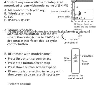
enter into code pairing state.2/Press UP & STOP button together for 10 seconds. 3/the fabric joys and code pairing completed.
